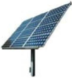
The Wattsun AZ-125 Gear Drive, azimuth tracker automatically tracks the sun by rotating the PV array about the pipe mast. Then it tilts for elevation position. The Dual-Axis Option enables it to capture virtually all the power the sun delivers. Compared to passive, tilt and roll trackers, azimuth trackers provide greater stability for large arrays. The corners do not protrude down towards the ground or stick up in the air to catch the wind. The bottom edge of the array always remains ...
